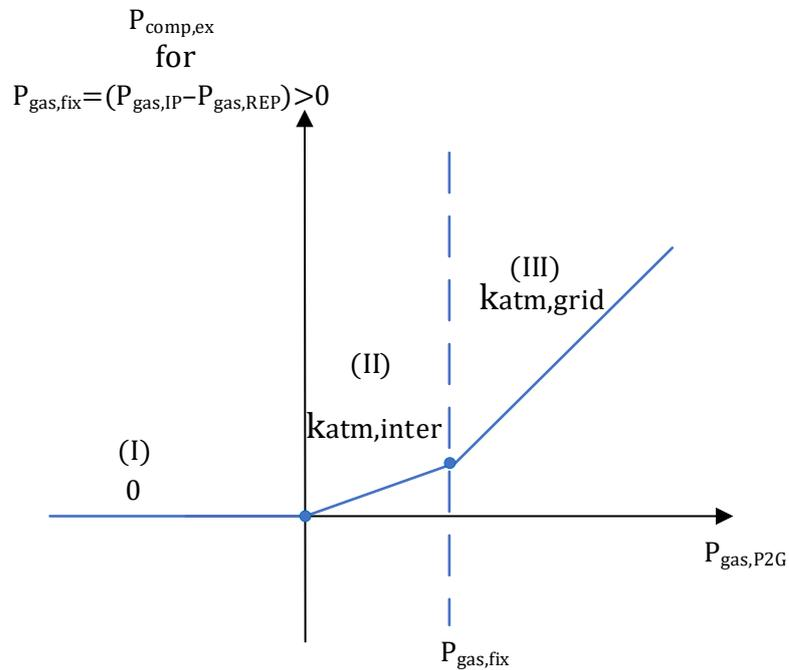
As it is shown in Fig. 7, compression characteristic has three partitions that can be represented with three conditions. Using (A1.70), accurate value of  $P_{comp,ex}$  is obtained when maximum of all three conditions is found:
