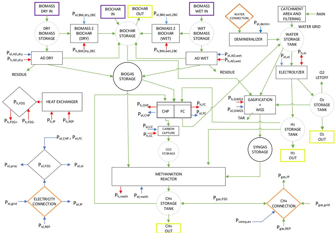
Without biochar part (Gasification + WGS, O<sub>2</sub> storage) the concept is reduced to “Biogas P2G”. For its heat and electricity production (CHP/FC), not only biogas but also a mixture of biogas and hydrogen is possible to use as feedstock. Exhaust CO<sub>2</sub> from the CHP can be captured and stored in the CO<sub>2</sub> storage. Instead of CHP, to produce heat and electricity, it is possible to use fuel cells (FC). In that case the only feedstock is hydrogen
