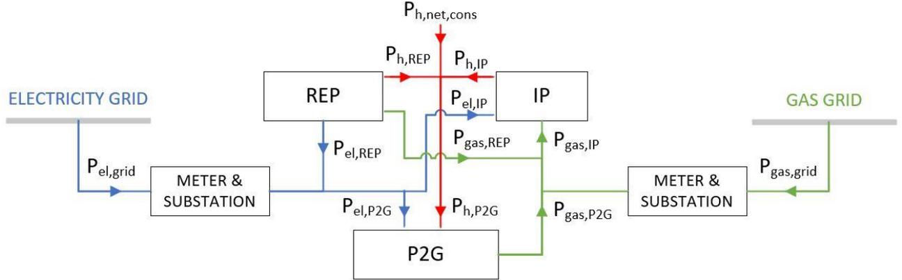
According to the electricity and gas grid connections as well as interconnections between P2G, REP and IP given in the scheme, the following equation system is obtained:
