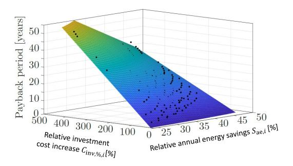
$PP_i = p_0 + p_1 \cdot S_{\text{ae},i} + p_2 C_{\text{inv},i} + p_3 \cdot S_{\text{ae},i} \cdot C_{\text{inv},\%,i}$
